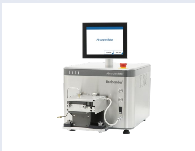
Mixer for characterization of industrial carbon blacks
