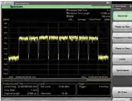
Spectrum of eight 100 MHz bandwidth carriers at 29 GHz center frequency
