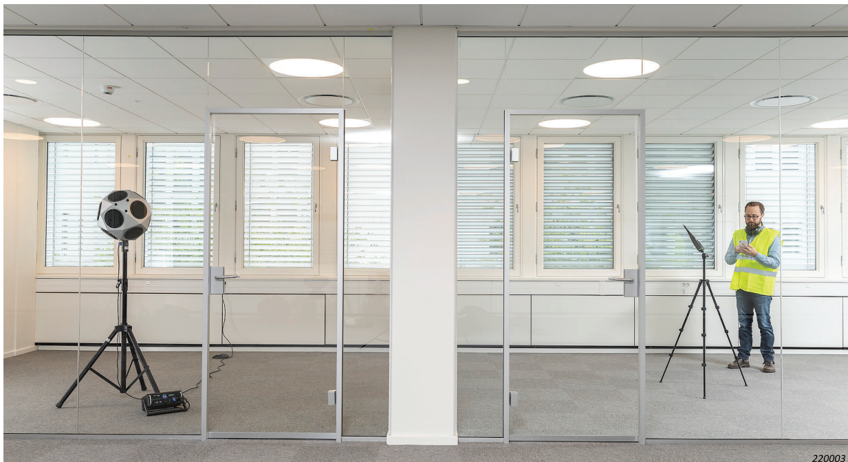
Fig. 2 Type 4292-L powered by HBK 2755 delivers the sound power required for sound insulation measurements
