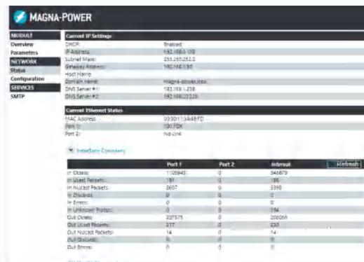
EtherNet/IP webpage hosted in Magna-Power's +EIP option with EtherNet/IP (+EIP) option.
