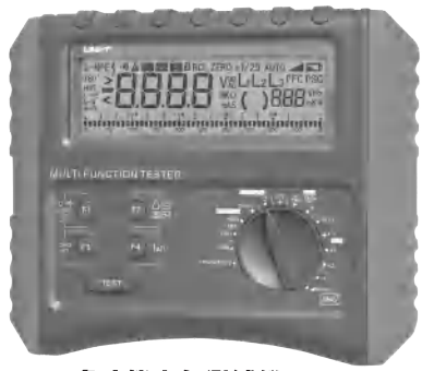
多功能电气测试仪 Multi-functional Electrical Measuring Instrument
