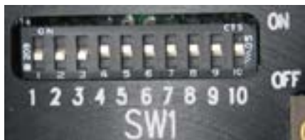
Figure 24. Ten-position DIP switch SW1.
