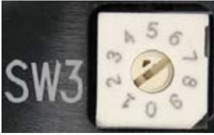
Figure 26. Ten-position rotary switch SW3.
