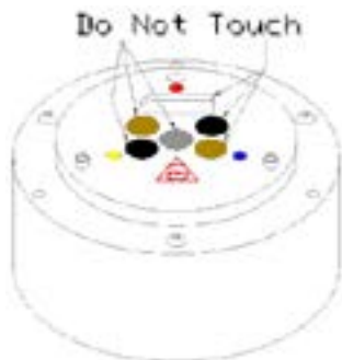
Figure 10. Electronics module sensor windows
