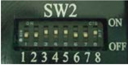
Figure 25. Eight-position DIP switch SW2
