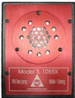
Figure 3. TL-1055 handheld test lamp (NEMA 1)
