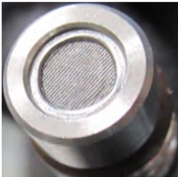
Example of clean orifice filter
