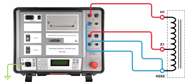
Connecting TRT to a single-phase autotransformer
