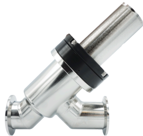
HV Inline valve, DN 25 ISO-KF, electro-pneumatic, PV 24 V DC, SS/FKM, "A"-dim. 107 mm
