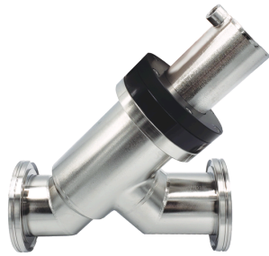
HV Inline valve, DN 80 ISO-K, electro-pneumatic, PV 24 V DC, SS/FKM, "A"-dim. 268 mm
