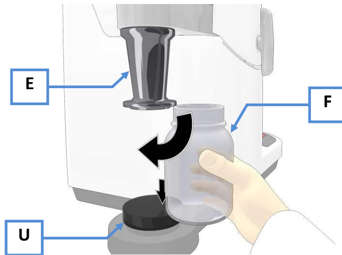
Fig. 9: Inserting the sample vessel
